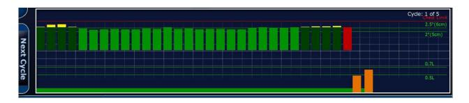
The compressions are showing a lot of bright green. Those are all very good. The dark green compression bars with a slight bit of yellow at the top indicate that rate and full recoil are correct but the depths were slightly beyond 2.5" or 6.4cm.
