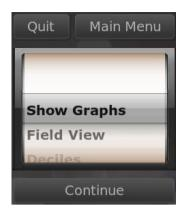
The second Roller Wheel is used to show a graph of the results you filtered from the group you defined. It also allows you to filter results by the Score Range. It has a slight brown color around the outer edge.
